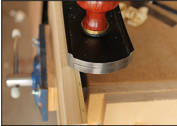
After locating and marking the high side, position the plane so the blade cuts only the high spot.
