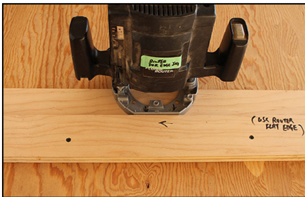
Make the base slightly larger and run the router against the fence to true the jig's edge.
