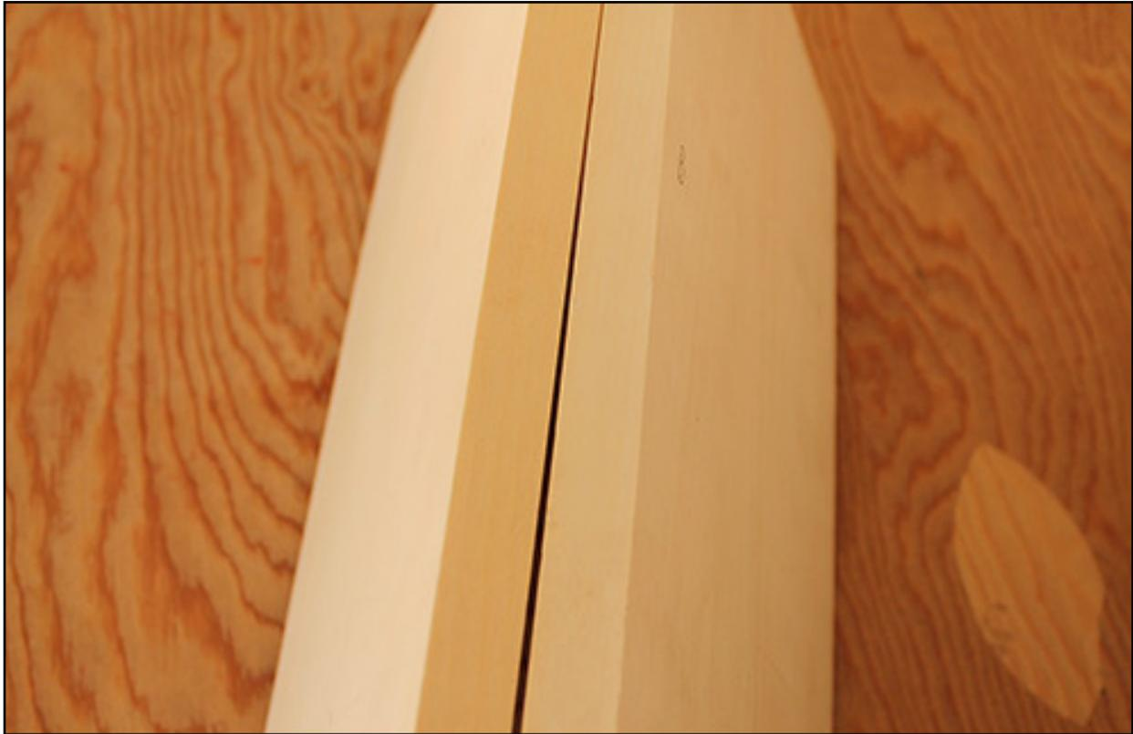
*Plane the edges as a pair and any bevel errors on either one will cancel out the other.*
