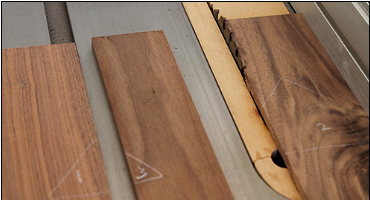
Rip the first edge of the next board and then flip the board to joint the second edge.
