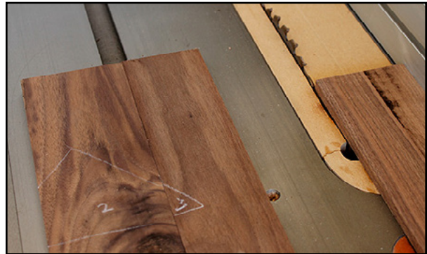
Flip the first board to rip the right edge on a left-tilt saw.
