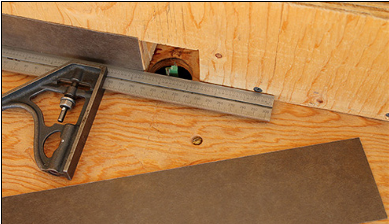
Using double-faced tape, secure a strip of plastic laminate to create an offset as the outfeed fence.
