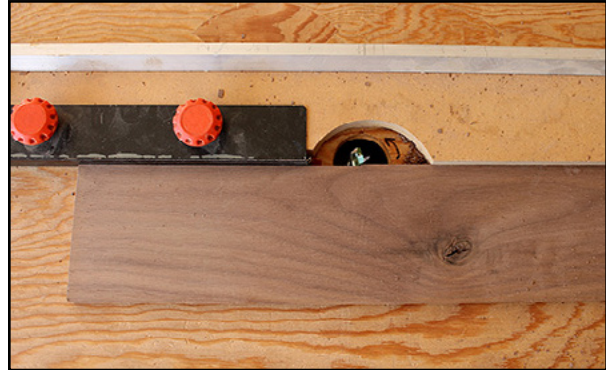
Similar to working with a jointer, apply pressure on the stock on the outfeed fence.
