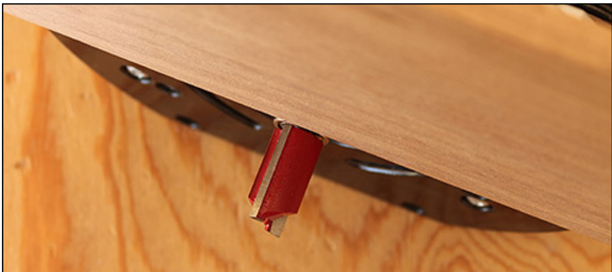
Set the pattern bit so that the bearing rides against the straightedge.
