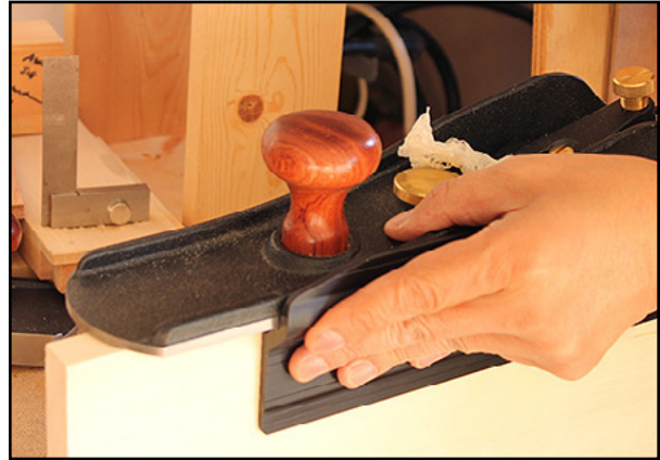
Press the fence against the workpiece as you push the plane forward.
